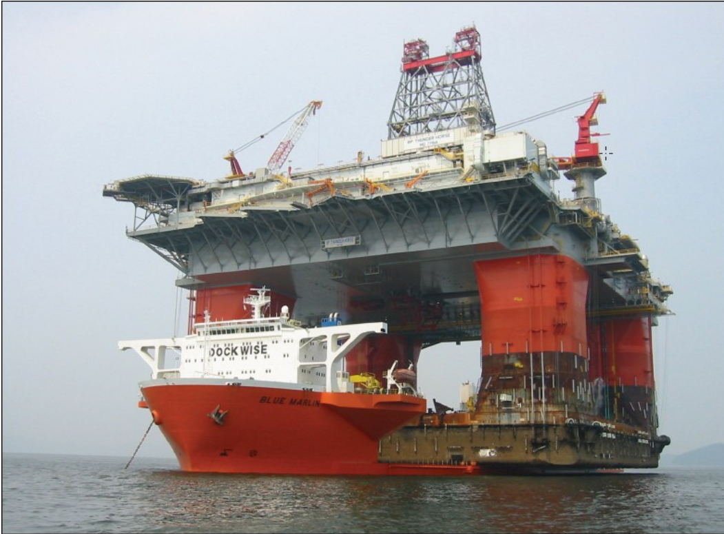
Figure 46: Thunder Horse Semi-Submersible Production Platform in transit to emplacement (Botros et al, © 2008 SPE. Reproduced with permission of the copyright owner. Further reproduction prohibited without permission.)
