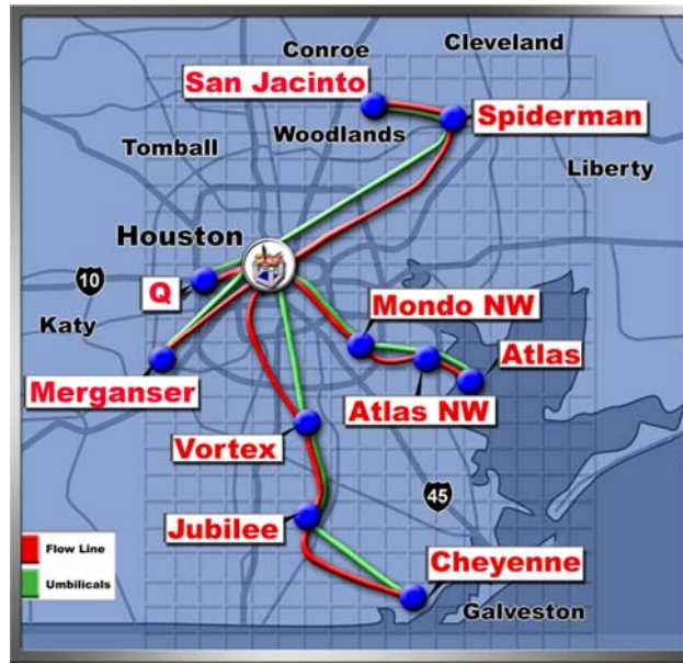
Figure 45: Independence facility gathering system overlaid on Houston area for scale 60 miles x 30 miles = 1800 square miles subsurface coverage area (Courtesy Anadarko Petroleum Corporation)
