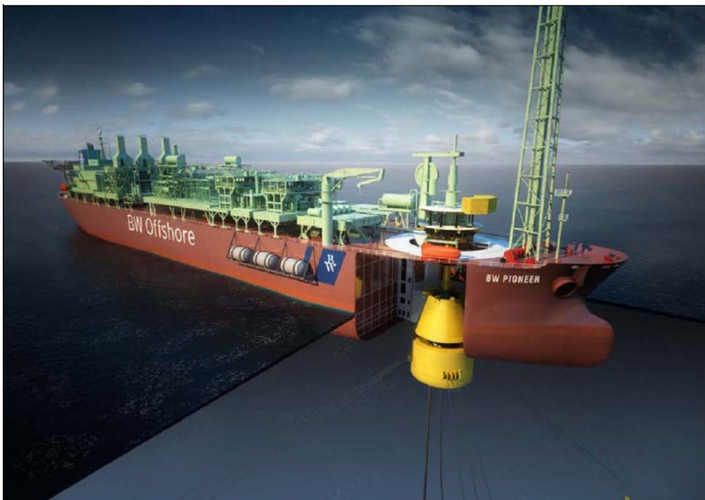
Figure 48: The BW Pioneer, a double-hulled tanker that will serve as the FPSO for the Cascade and Chinook developments. (Depiction courtesy of Petrobras) (From OCS Report MMS 2009-016)
