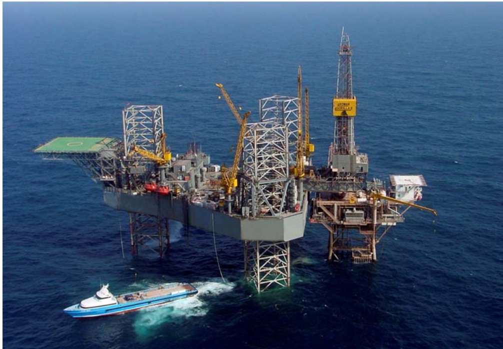
Figure 30: Rowan Gorilla VI Cantilevered Jack-up Drilling Rig (Rowan Companies, Inc.). Note cantilevered section extended over the top of a platform
