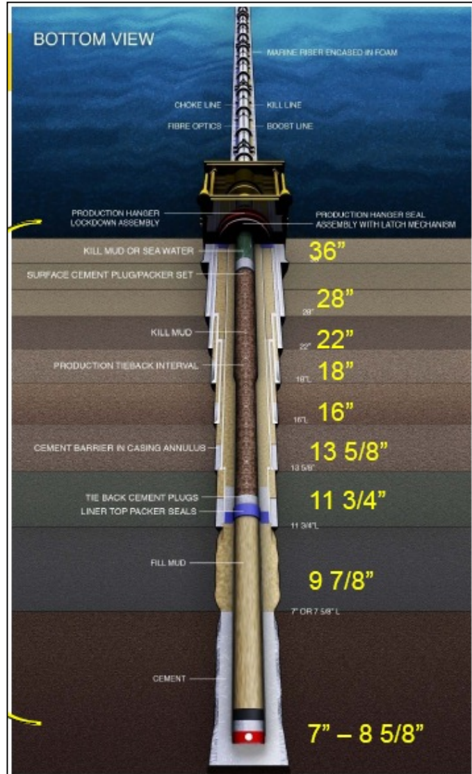
Figure 6. Examples of changes in drill casings during downhole well development. (Leimkuhler, 2010).
