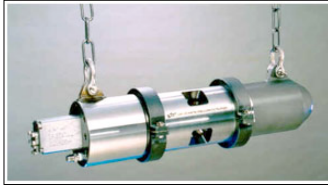
Figure 3. Marine seismic-acoustic airgun suspended on tow chains (SeaSCAN, 2010). The gun uses pressurized air to drive a piston from right to left to generate sound waves that exit the left end of the device. The overall length of the gun is about three feet.
